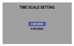
NOTE: Cycling 12VDC power will reset the time scale to 4 SECONDS.
