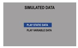
NOTE: Simulated data is disabled when a pressure sensors assembly is attached.
